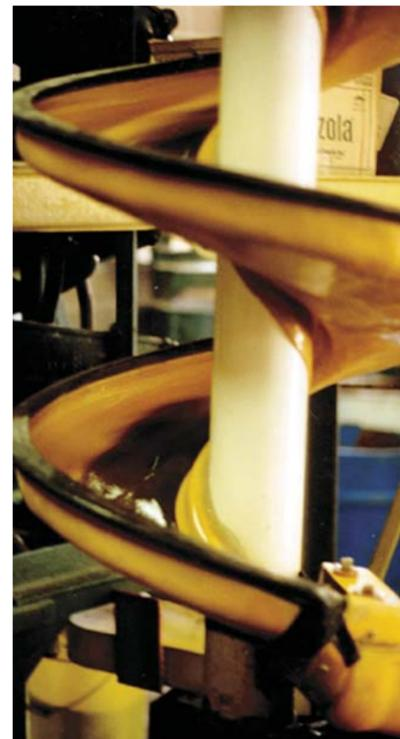
Spirals separate different density minerals using centrifugal force (left). Oil sand mining uses large-scale shovels and trucks (right)
